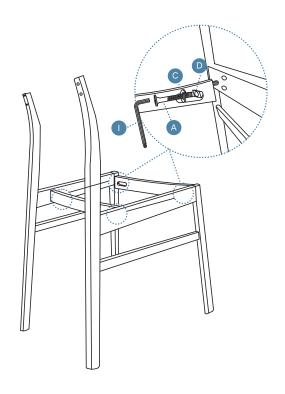
Attach assembled frame together as shown and secure with 4 x screws (A), 4 x spring washers (C) and 4 x screw pins (D). Tighten with an Allen Key (I).
