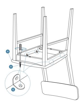
Attach 1 x seat (4) to assembled frame and secure with 4 x brackets (G) and 8 x screws (H). Tighten with a screwdriver.
