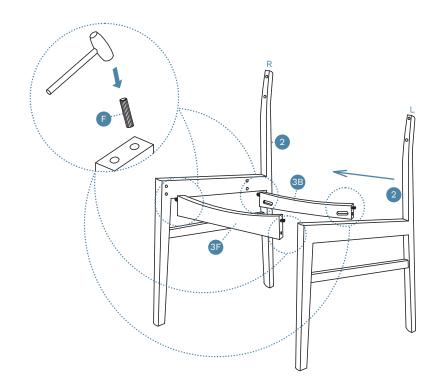
Attach 4 x dowels (F) to 2 x strechers (3F - Front) and (3B - Back) and 2 x legs (2) as shown. Panels number 3 are marked F and B, F is the panel for the front of the chair and Panel B is for the back of the chair.
